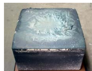
Fig. 5.9 400 kg ingot produced in Integrated Project Crystal-Clear. Source: Deutsche Solar, Germany
