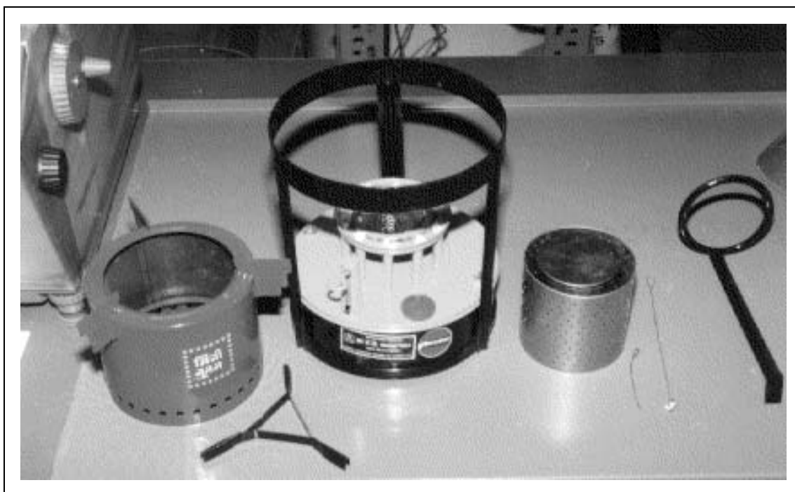
Figure 7.4: Photo of a superior wick stove and its individual parts (LAUTERBACH/SCHNAITER 1995)
